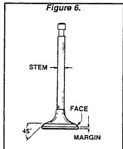
NOTE: Proper lapping of valves and valve seats will remove grinding marks and ensure a good seal between the valve and its seat. Be sure to clean lapping compound from the valve seats and faces.
